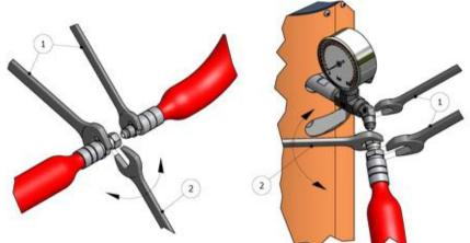
Figure 3. Hose coupling method
